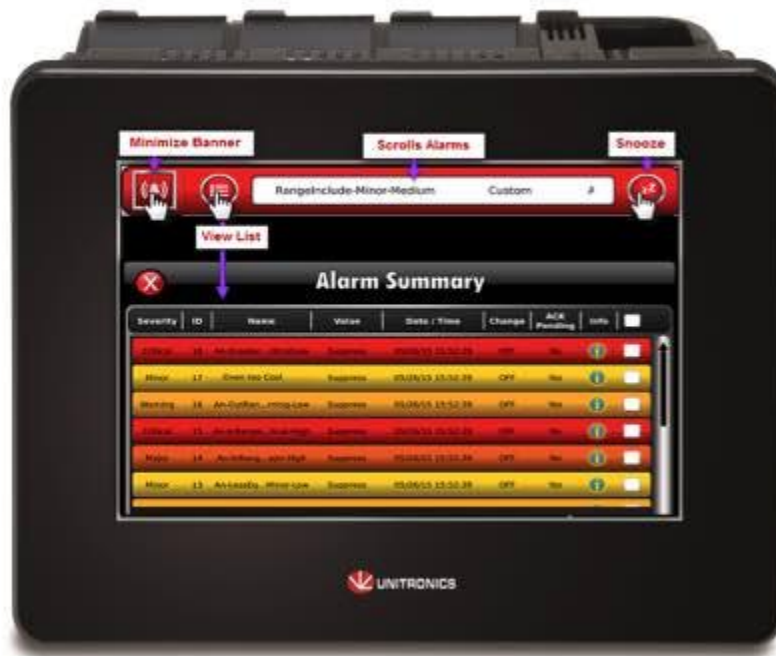
Fig.5.5 Alarm Management system PLC HMI product
