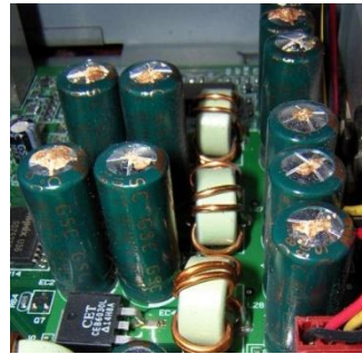
Faulty capacitor unit with bulging body
