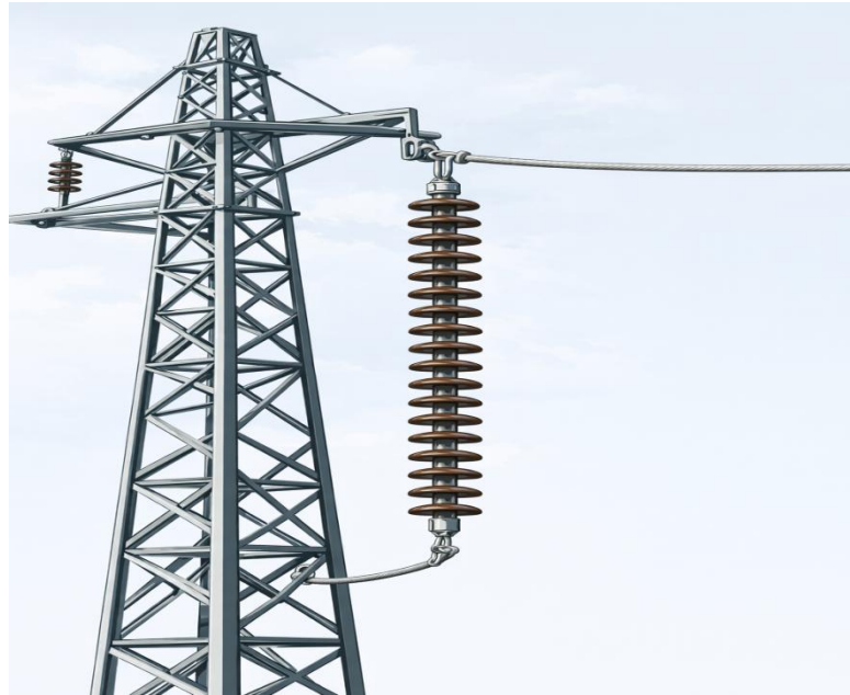
Fig. A vertical tower with a string of round discs hanging and supporting a conductor.
