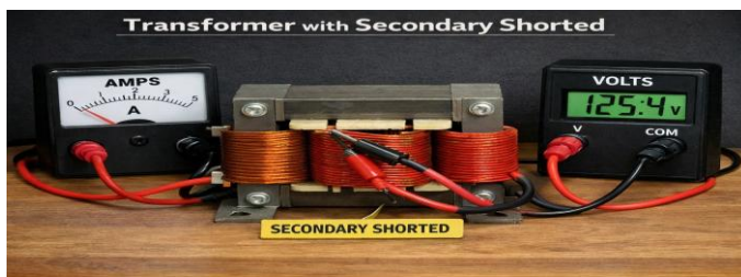
Fig.3.3.8.a.:Transformer with secondary shorted and voltmeter, ammeter on primary side.
