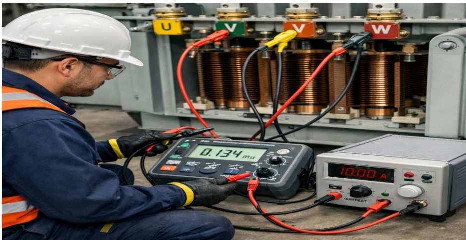
Fig.3.2.b. Technician measuring winding resistance using test instruments.
